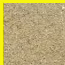
SAND Particle size 0.2 mm to 2 mm
